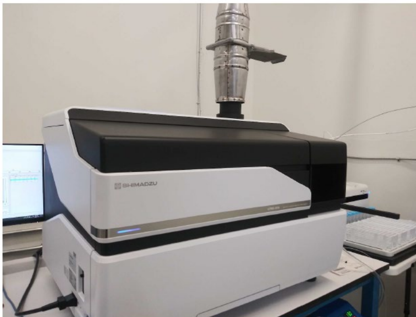
Figure 1. Inductively Coupled Plasma Mass Spectrometer (ICP-MS) from Shimadzu Scientific. Picture taken at Confidence Analytics in Redmond Washington on July 6th, 2020. The unit can test up to 20 samples per hour for heavy metals analysis. This unit alone has enough capacity to test over 10,000 samples per month, giving it plenty of capacity to meet future demand. Confidence Analytics will be submitting a validation report to the RJLee Group in the coming weeks.
