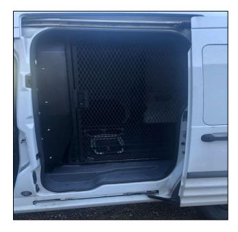
Below: Example of a secondary cage built within the interior of a locked vehicle:
